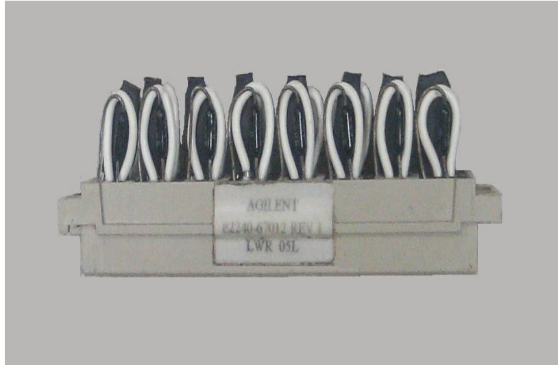
Figure 4-14 CEDGN Loopback Connector (E2240-67012) CEDGN test load module for E6175A, U7177A, and N9377A
