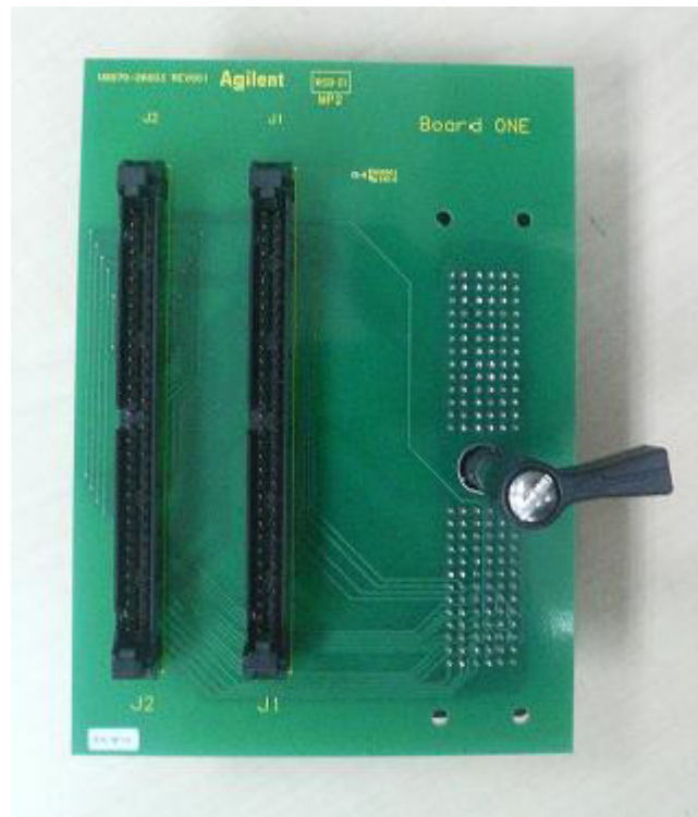
Figure 4-7 CEDGN Board #1 (U8970-66603 PCA- Diagnostic Number 1)
