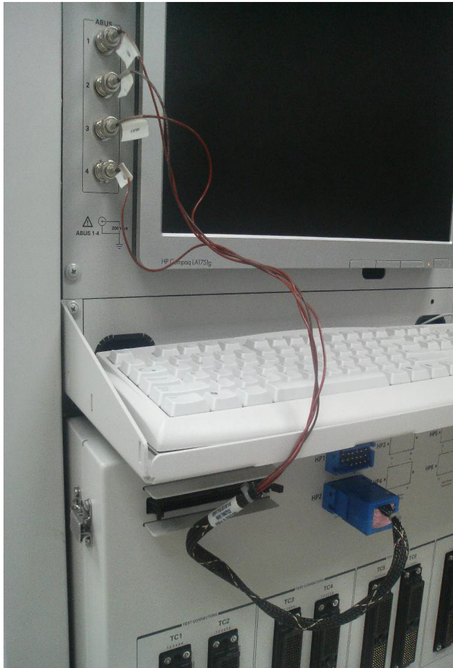
Figure 3-4 Installing 8-Ch Heavy Duty Card diagnostic cable E6170-61618 on HP2 and BNC connectors to Abus1, Abus2, Abus3 and Abus4.
